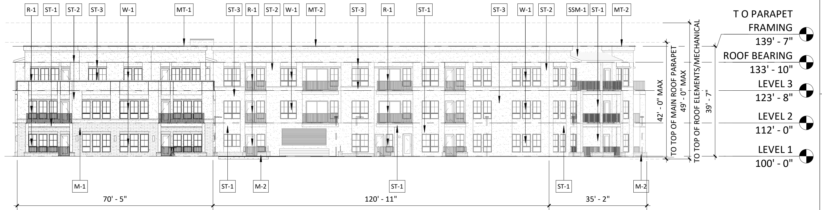
3 NORTH ELEVATION - DRB B/W A.21.vd 1" = 20'-0"
