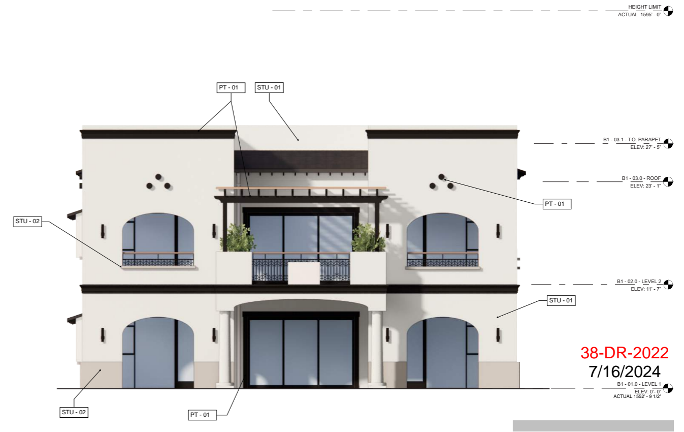
2 BUNGALOW 1 - SOUTH ELEVATION 1/4" = 1'-0"
