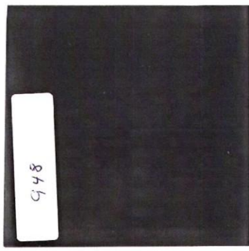
SGL-1 SPANDREL GLASS: BLUR TINTED W/ MED. GRAY OPACIFIER TO MATCH VIRACON #948
