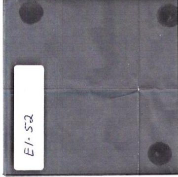
VGL-2 VISION GLASS: LIGHT BLUE-TINTED INSULATED GLAZING TO MATCH VIRACON VE1-52 or CARDINAL LoE-240
