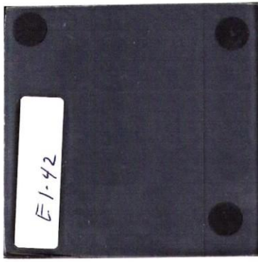
VGL-3 VISION GLASS: MED. BLUE-TINTED INSULATED GLAZING TO MATCH VIRACON VE1-42
