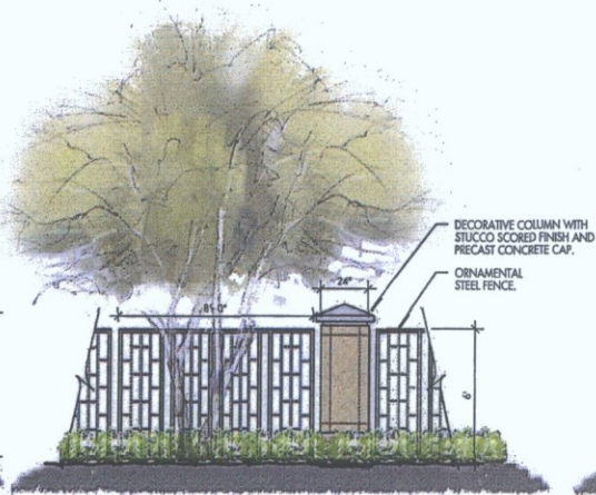
FULL VIEW /POOL FENCE WITH COLUMN
