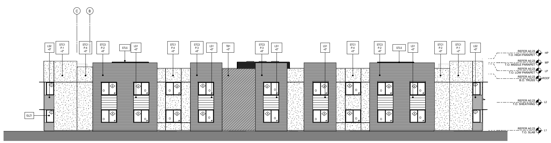
1 ELEVATION - BUILDING D.1 - EAST AZ 10 1/8" = 1'-0"
