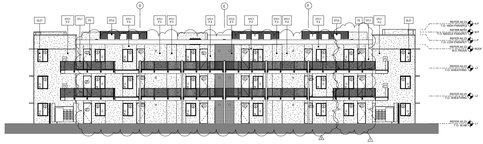
2 ELEVATION - BUILDING A.2 - COURTYARD SOUTH A2.02 1/8" = 1'-0"
