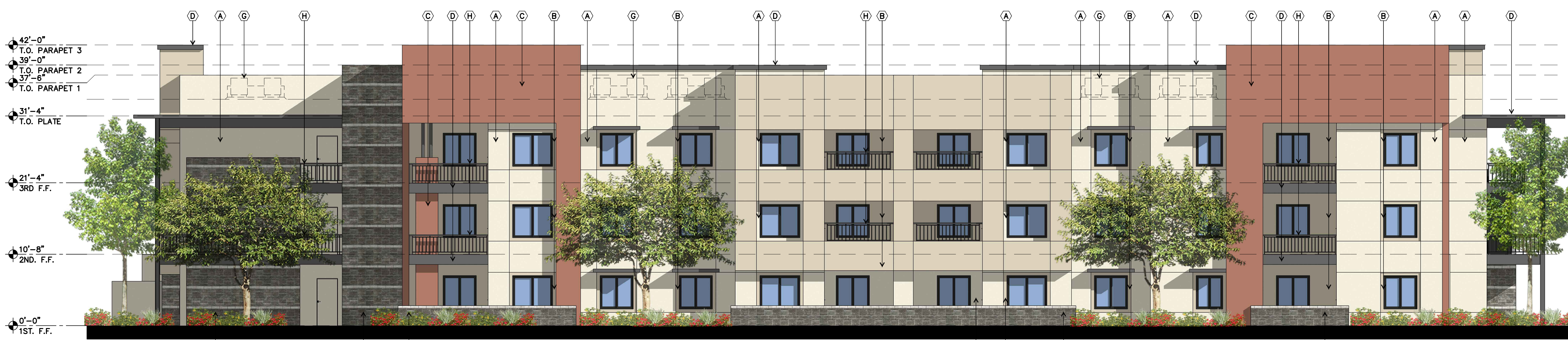
2 BUILDING 3 - REAR ELEVATION SCALE: 1/8" = 1'-0"
