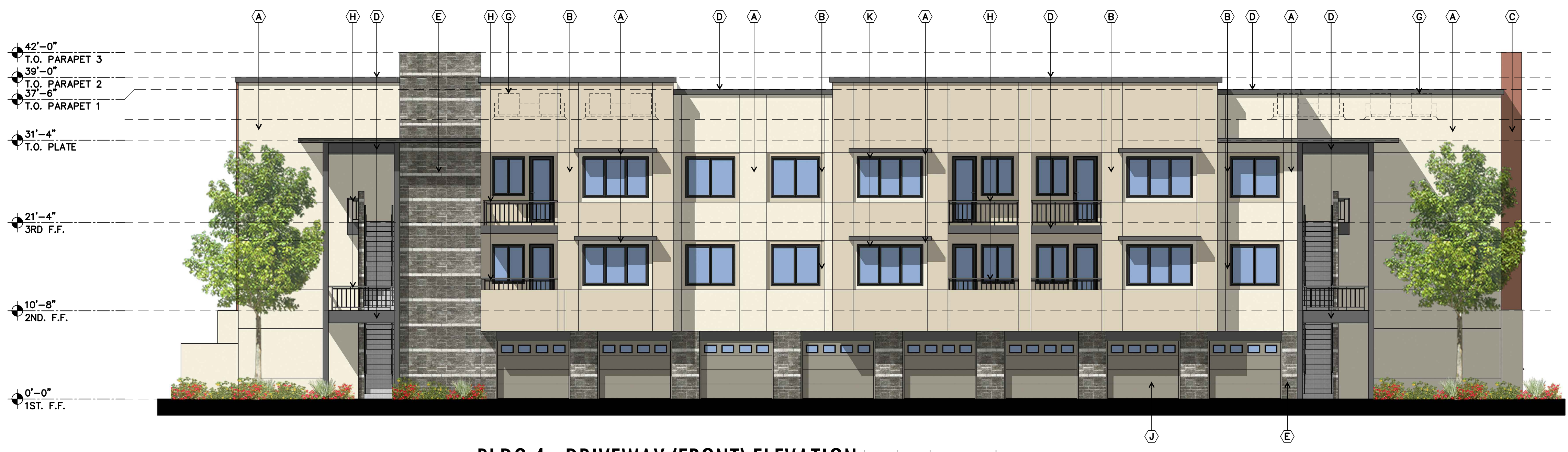
1 BLDG 4 - DRIVEWAY (FRONT) ELEVATION SCALE: 1/8" = 1'-0"
