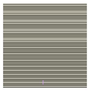
3" EIFS with Horizontal 1" deep groove pattern to match Villa stair screening Colors: EIFS Color 1 & 2 (as shown on elevations)
