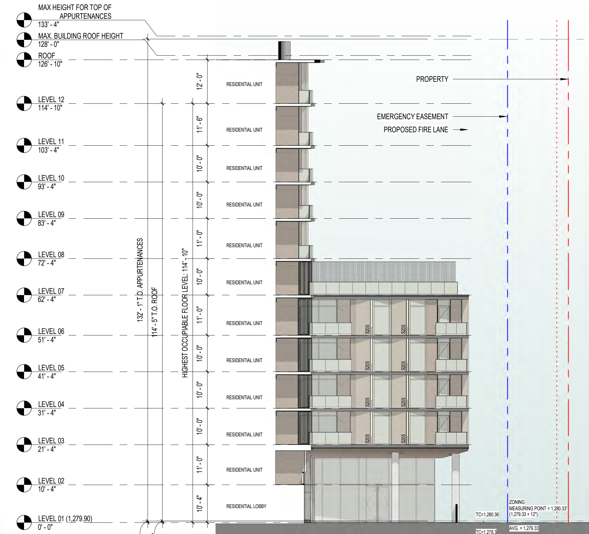
3 COURTYARD NORTH WEST ELEVATION (DRB) 1/16" = 1'-0"
