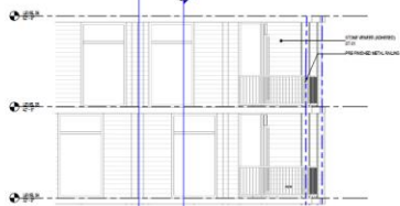
1 ENLARGED ELEVATION - WEST SANDSTONE
