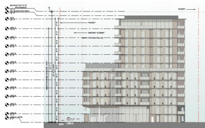
2 SOUTH EAST ELEVATION (DRB) 1/16" = 1'-0"
