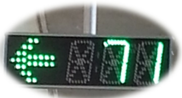
Signs have built in light meters and auto adjust.
