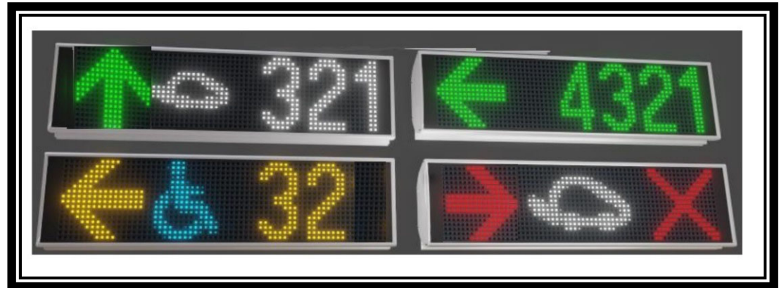
New signs rotate through Standard, ADA and EV
