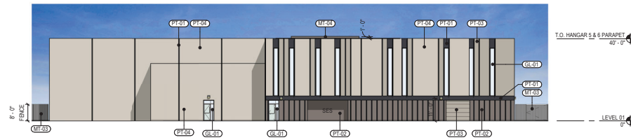
4 DRB - ELEVATION - HANGAR 05 & 06 - SW SCALE: 1" = 20'-0"
