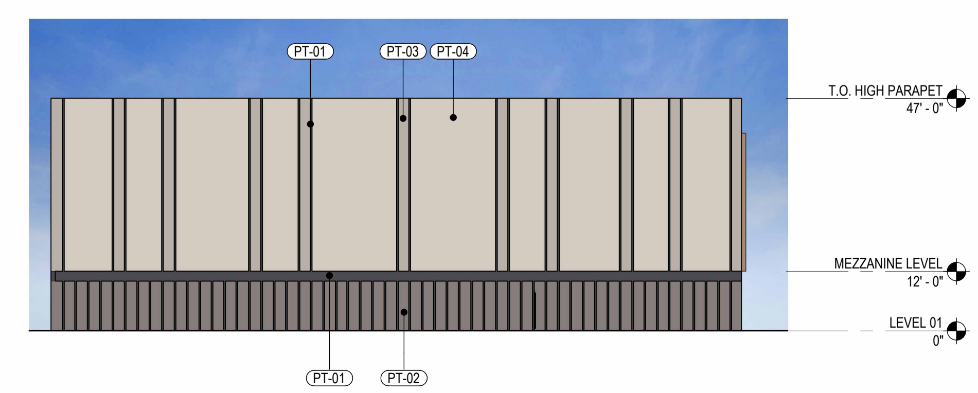
1 DRB - ELEVATION - HANGAR 03 & 04 - NW SCALE: 1" = 20'-0"
