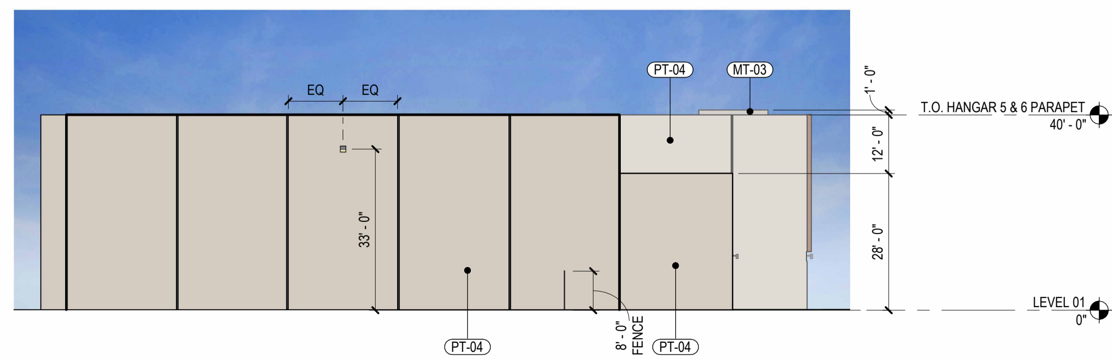
1 DRB - ELEVATION - HANGAR 05 & 06 - NW SCALE: 1" = 20'-0"
