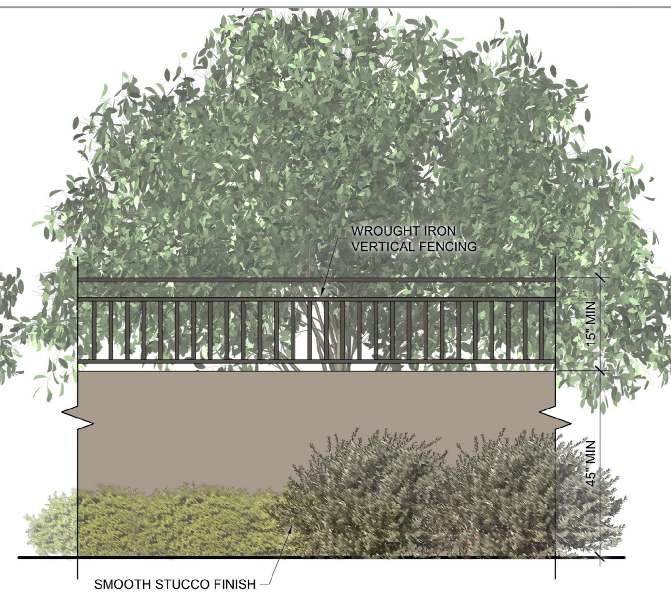
3 Partial View Wall - Perimeter and On-Site SCALE: 1/2" = 1'-0"
