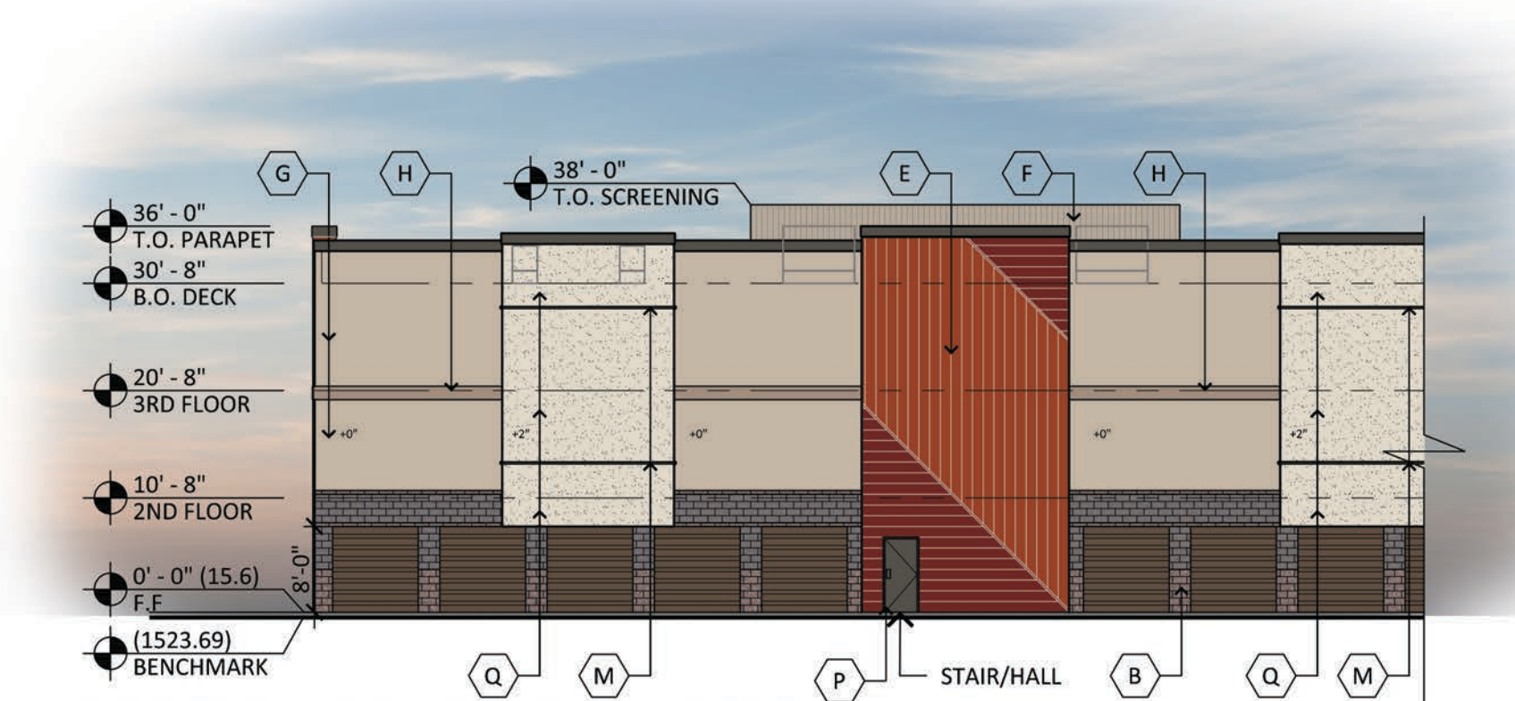
PARTIAL SOUTH ELEVATION
