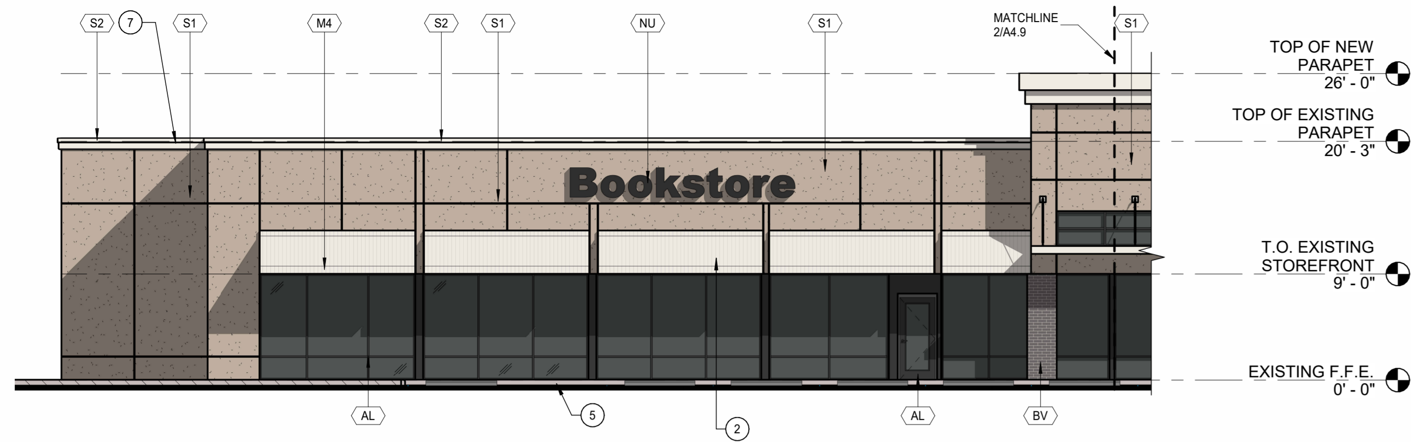
1 BLDG. A ELEVATION - NORTH SIDE (NEW) 1/8" = 1'-0"
