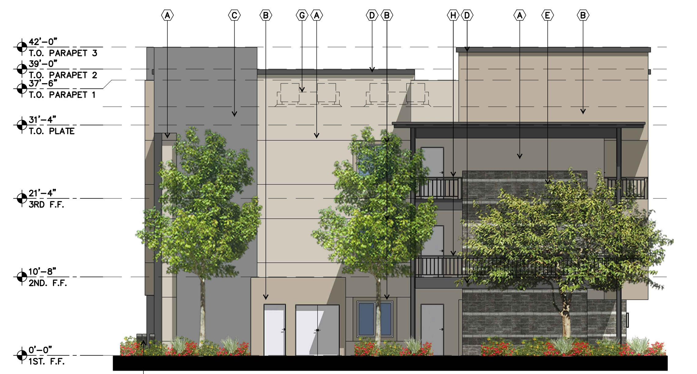
4 BUILDING 3 - LEFT SIDE ELEVATION SCALE: 1/8" = 1'-0"
