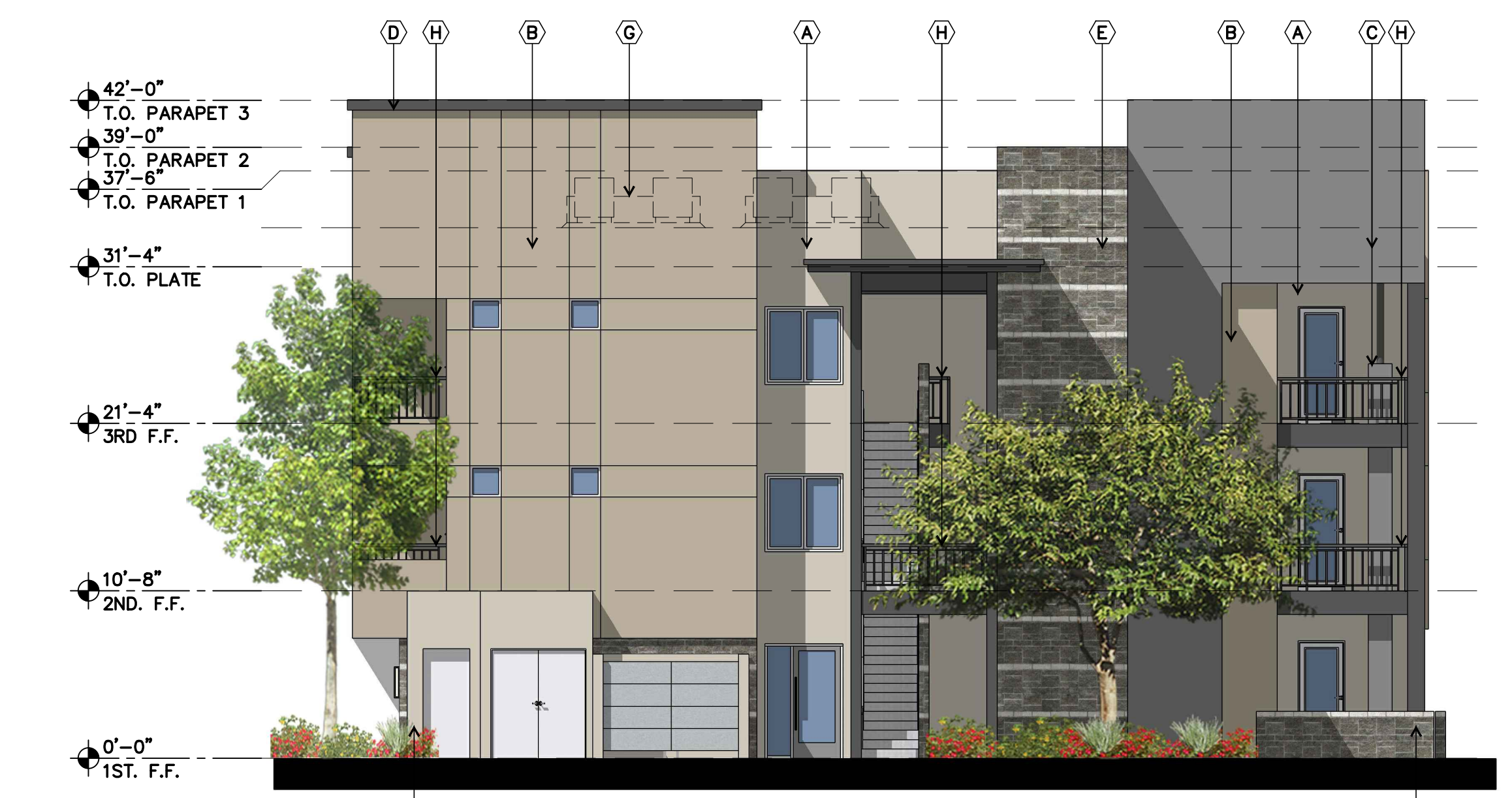
3 BUILDING 3 - RIGHT SIDE ELEVATION SCALE: 1/8" = 1'-0"
