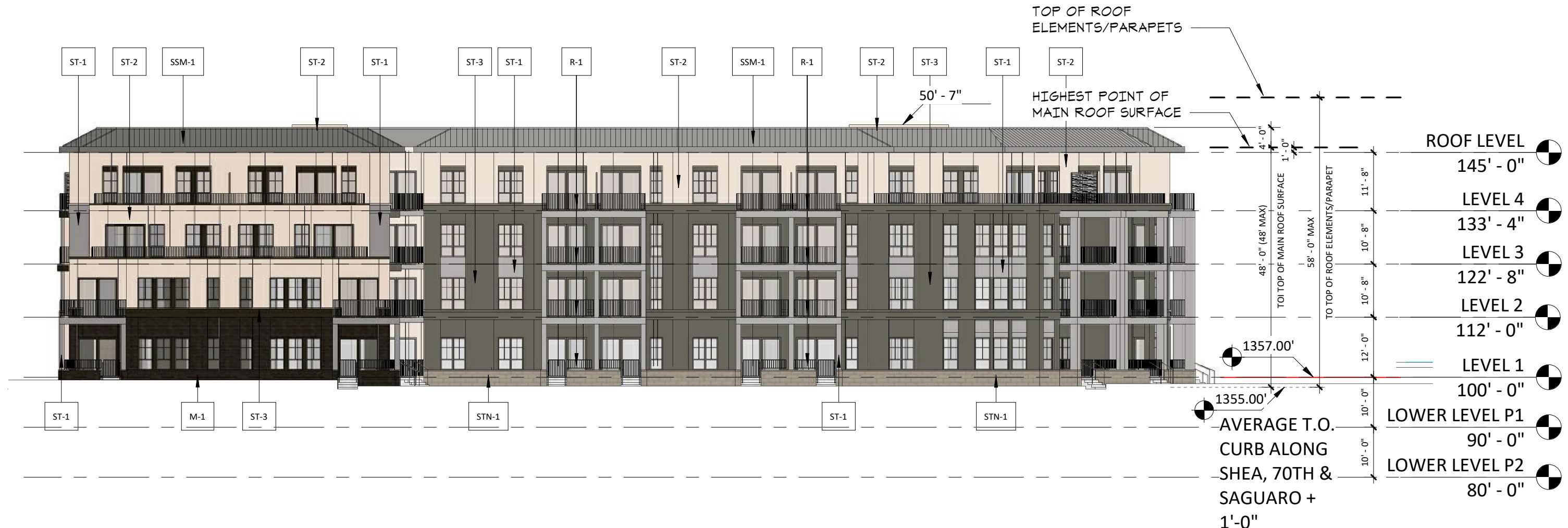
4 NORTH ELEVATION A.21.va 1" = 20'-0"
