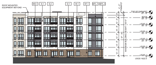
5A NORTH COURTYARD - NORTH ELEVATION A2.1 1" = 20'-0"
