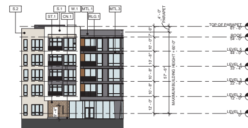
7D ENTRY PLAZA - EAST ELEVATION A2.2 1" = 20'-0"
