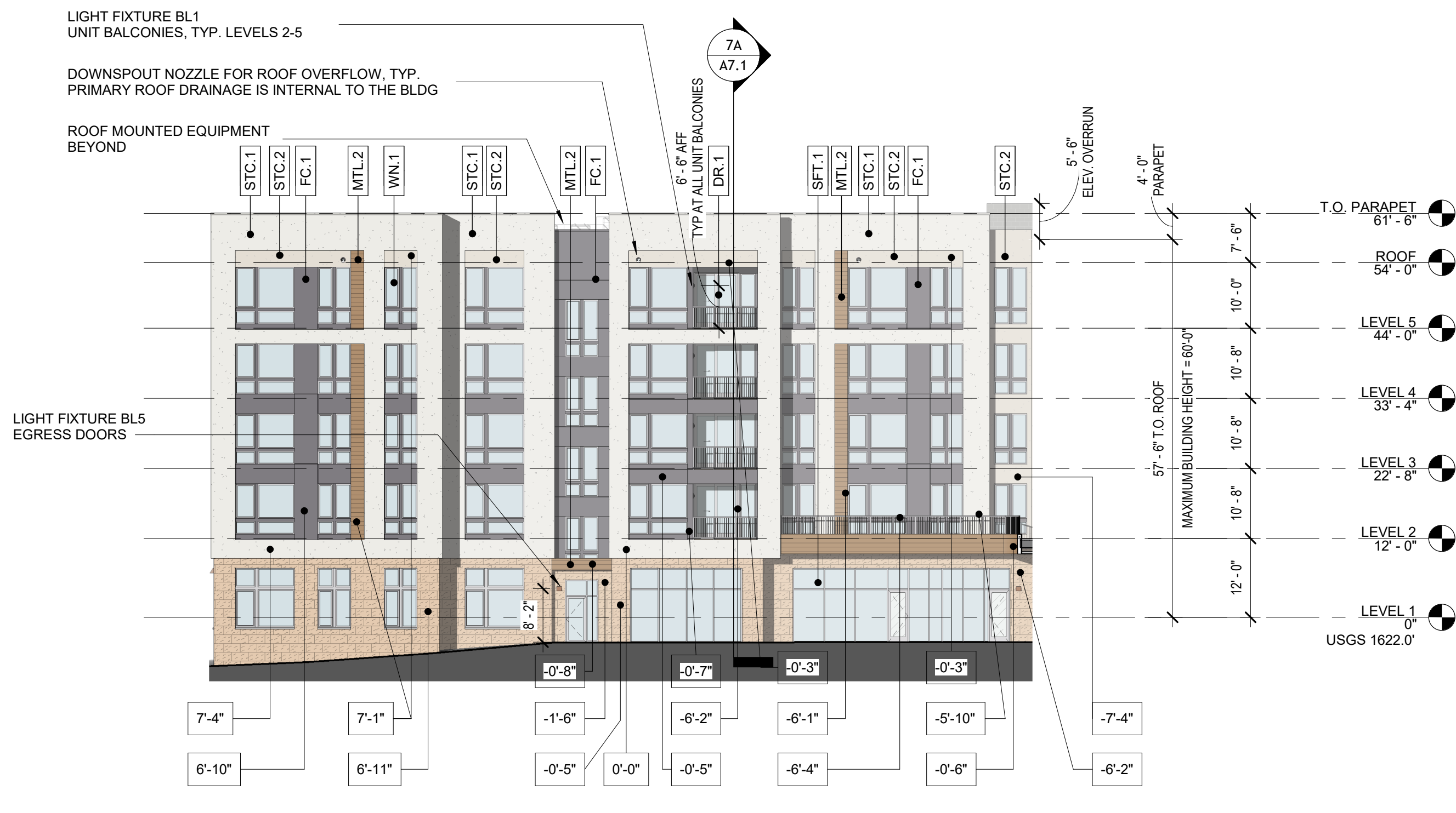
5E SOUTH COURTYARD - SOUTH ELEVATION A2.2 1/16" = 1'-0"
