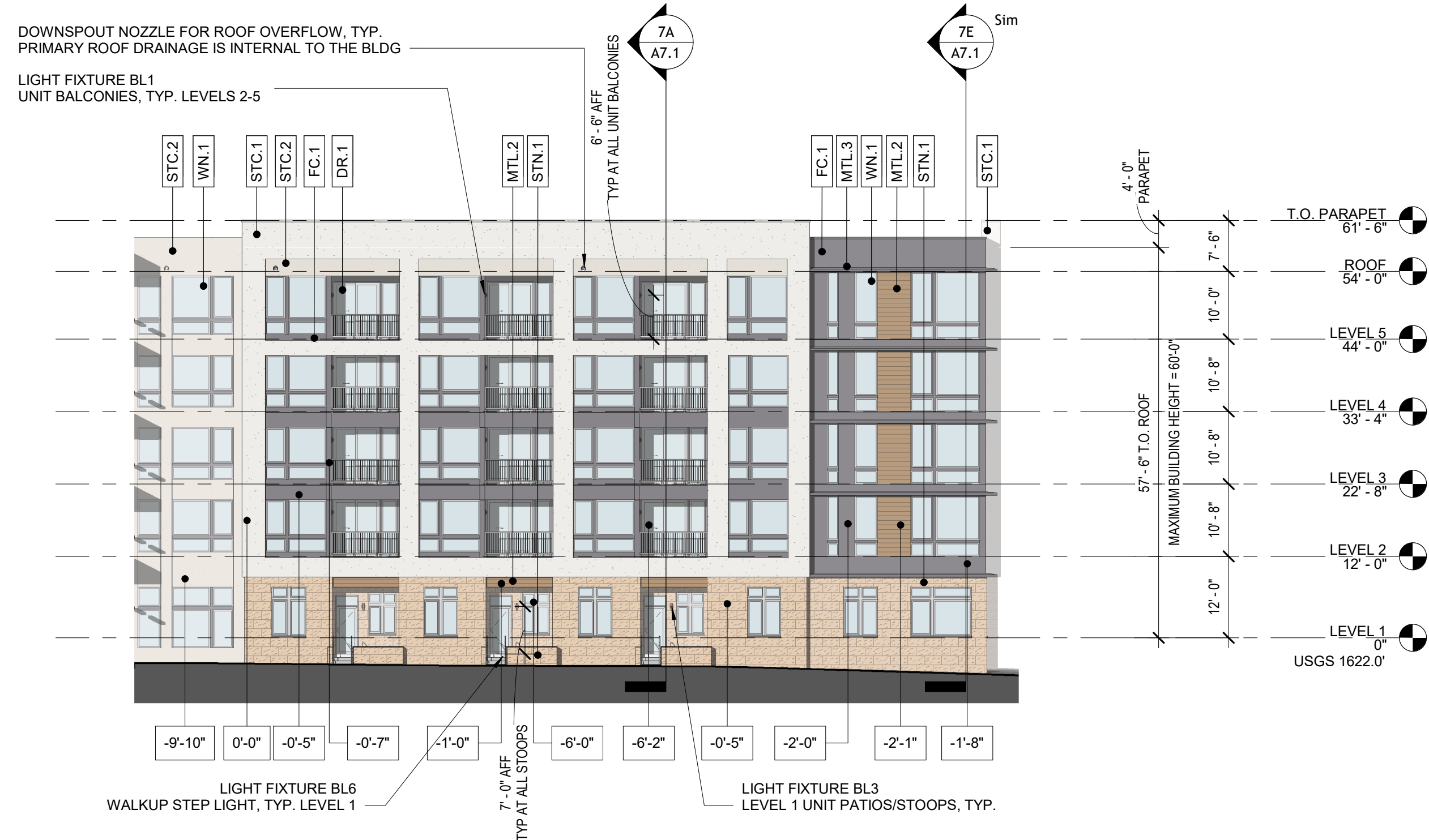
5A SOUTH COURTYARD - NORTH ELEVATION A2.2 1/16" = 1'-0"
