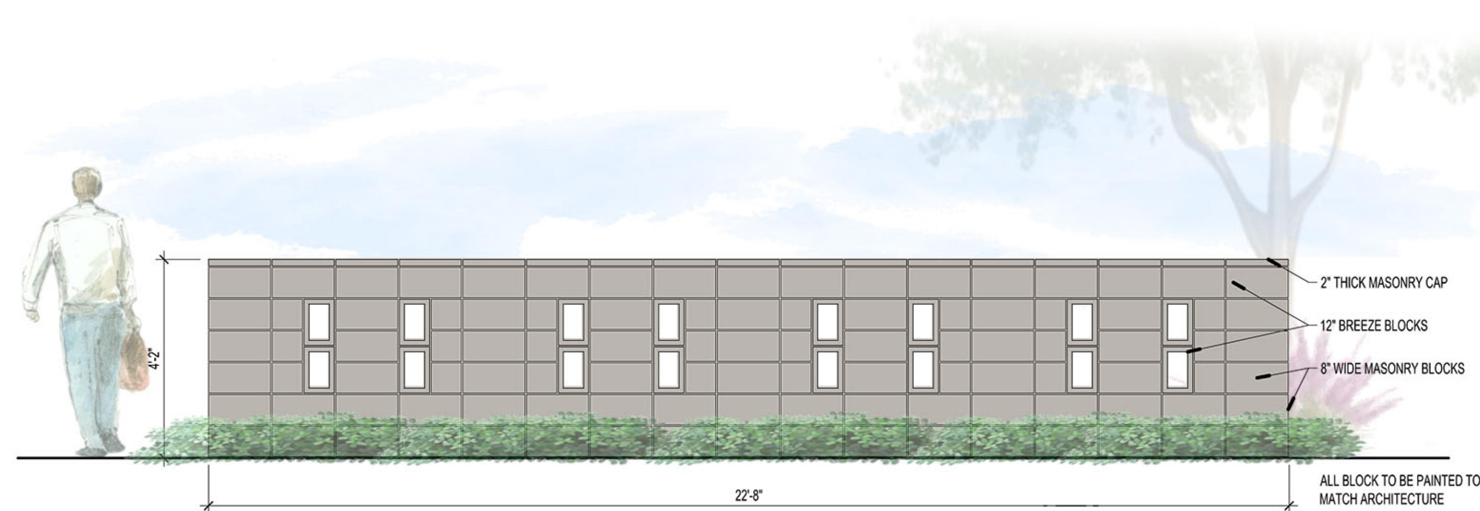
E COURTYARD SCREEN WALL SCALE: 1/2" = 1'-0"
