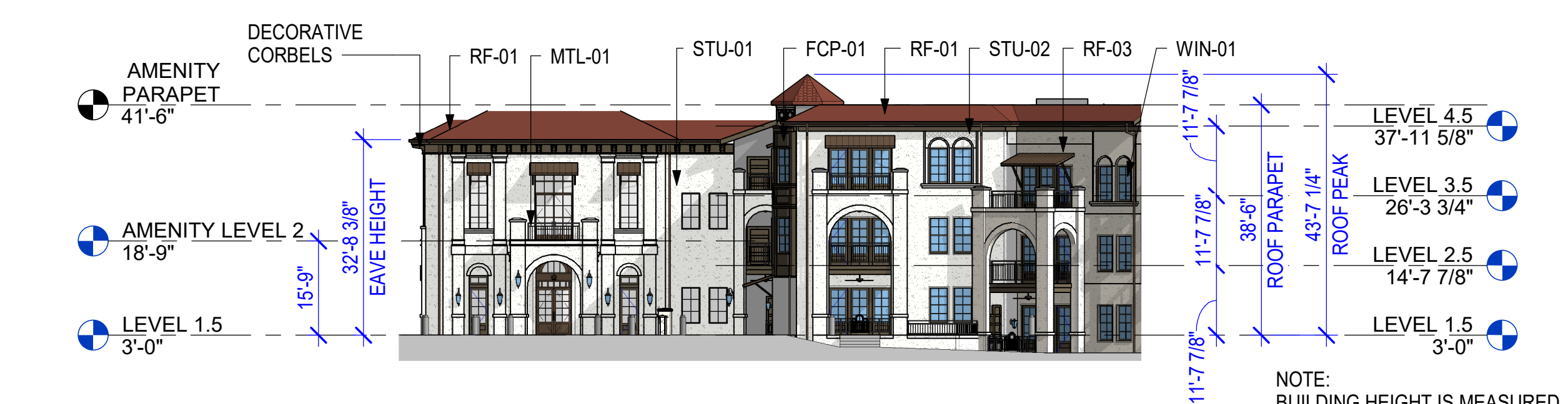
1 WEST ELEVATION - AMENITY BUILDING - DRB 1" = 20'-0"
