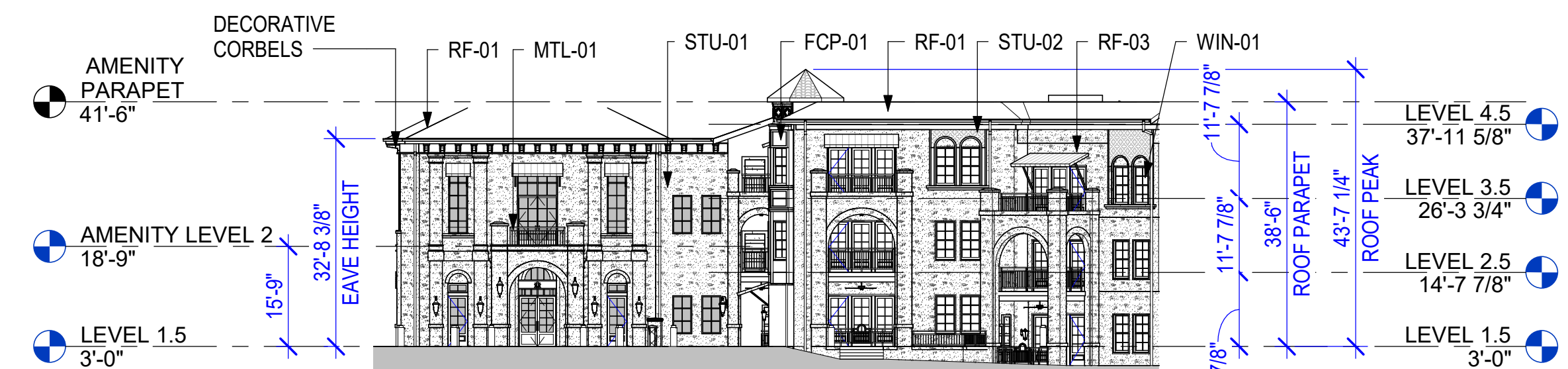
1 WEST ELEVATION - AMENITY BUILDING - DRB - B&W 1" = 20'-0"
