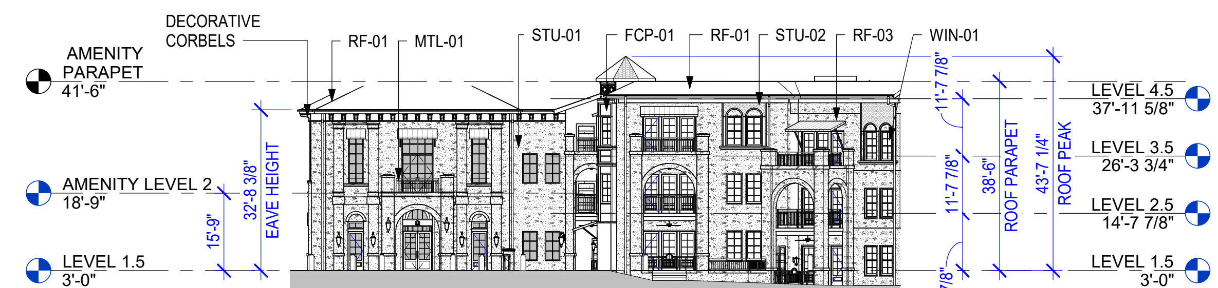
1 WEST ELEVATION - AMENITY BUILDING - DRB - B&W 1" = 20'-0"
