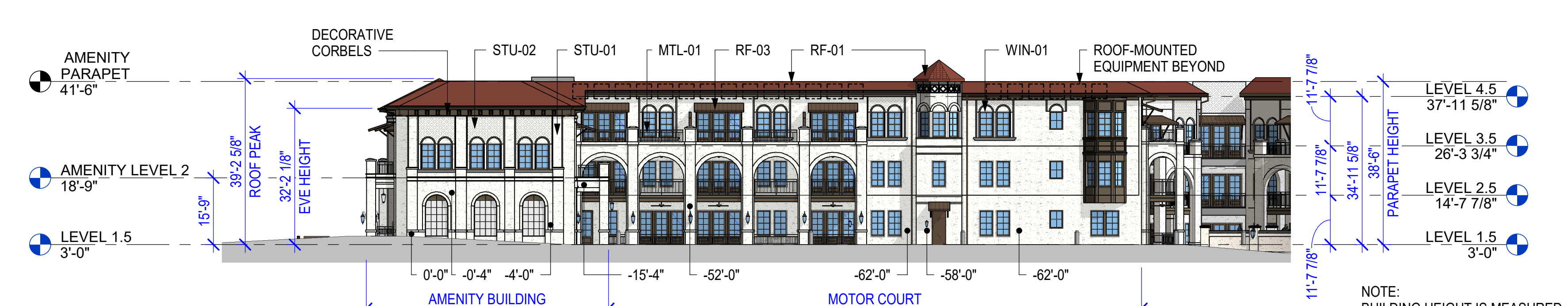
3 NORTH ELEVATION - AMENITY BUILDING - DRB 1" = 20'-0"
