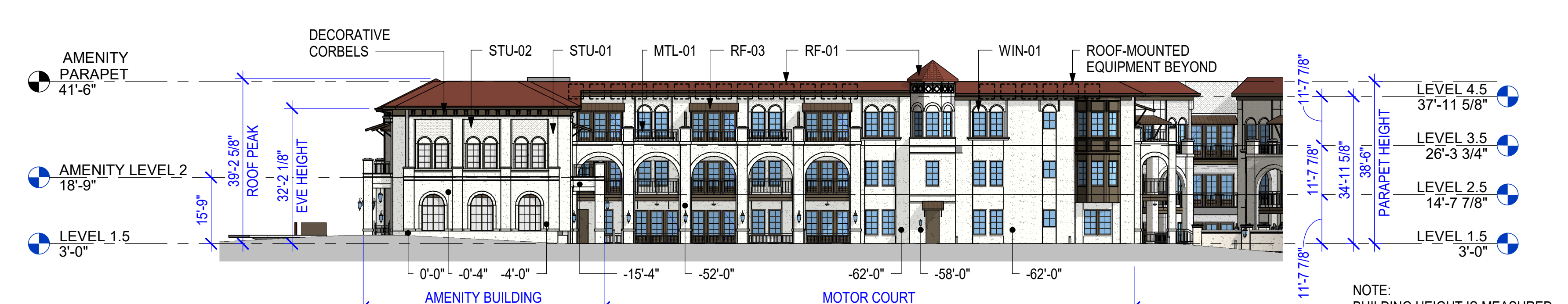
3 NORTH ELEVATION - AMENITY BUILDING - DRB 1" = 20'-0"
