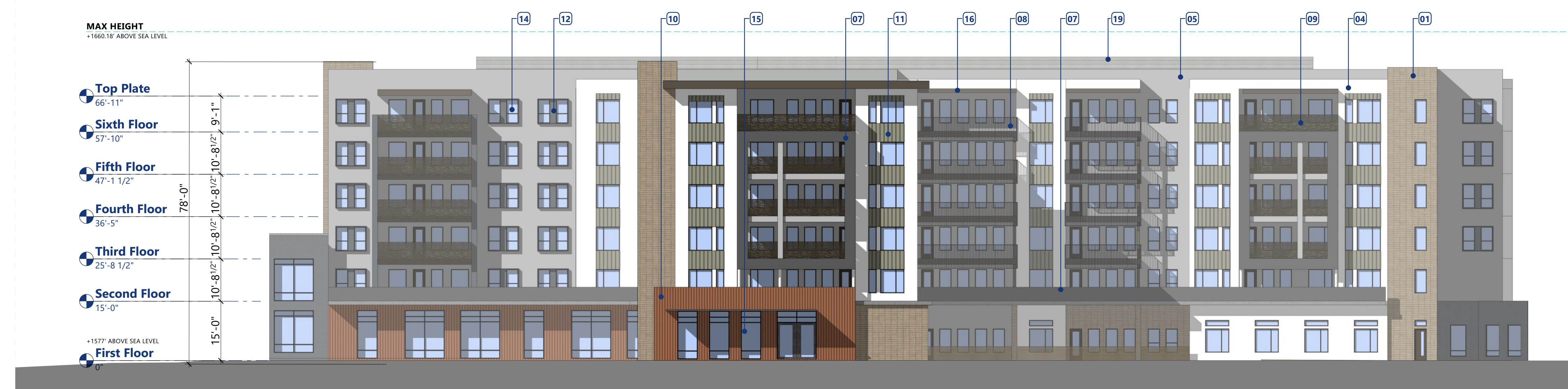
07 BUILDING RB 1.2 - ELEVATION 01 SCALE: 1/16" = 1'-0"
