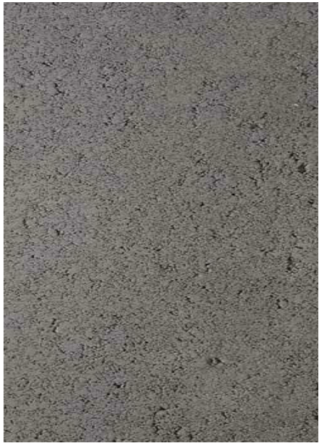
CMU-1 DESCRIPTION: 8' X 8' X 16' GROUND FACE CONCRETE MASONRY LOCATION: EXTERIOR SITE WALLS MANUFACTURER: RCP BLOCK PRODUCT: PRECISION BLOCK COLOR: CHARCOAL GREY
