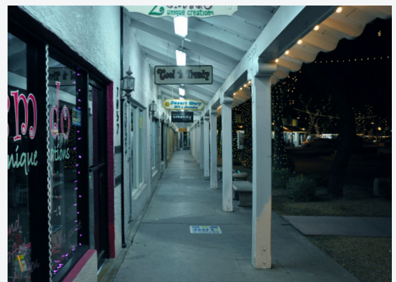
DISCOURAGED - Not all types of lighting are suitable for pedestrian areas. The use of unfiltered fluorescent lighting is strongly discouraged.
