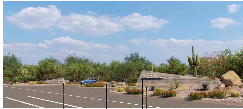
RAMMED EARTH WALLS 8' 2' WILDCAT HILL LARGE BOULDERS RECLAIMED FROM ON-SITE ANCHOR THE WALL RAMMED EARTH ENTRY SIGN SIGN - STEEL CUT LETTERING SITS ATOP A STEEL PLATE EMBEDDED INTO THE EARTHEN WALL
