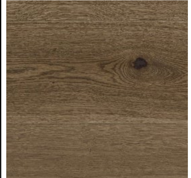
④ WD-1 - WOOD BEAMS & COLUMNS SPECIES: OAK, STAINED AND TREATED TO MATCH SAMPLE
