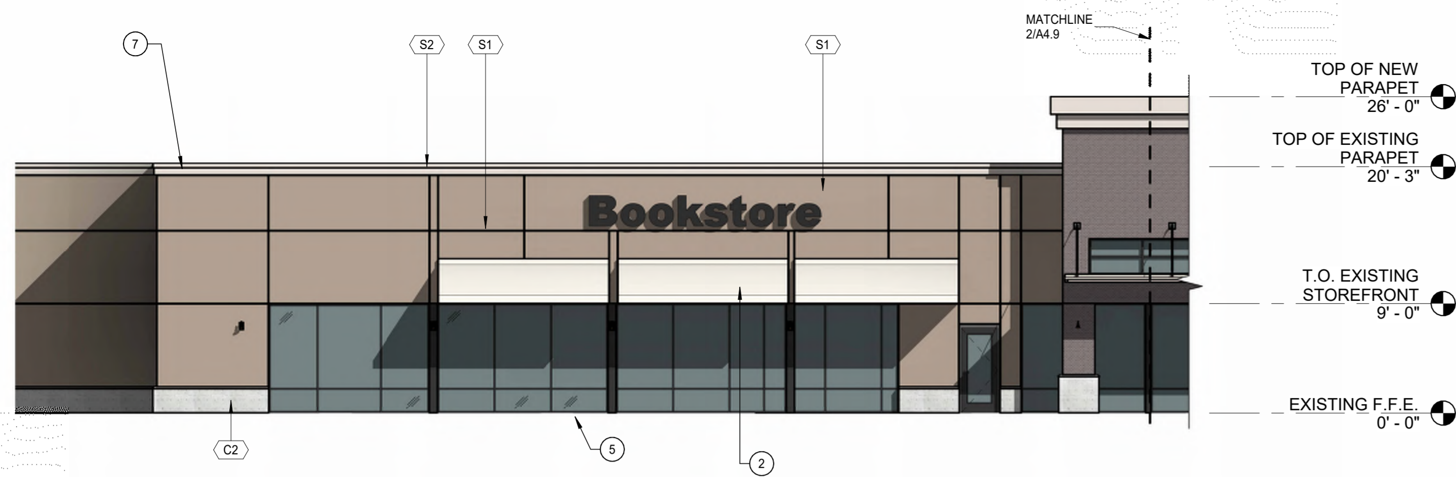
1 BLDG. A ELEVATION - NORTH SIDE (NEW) 1/8" = 1'-0"
