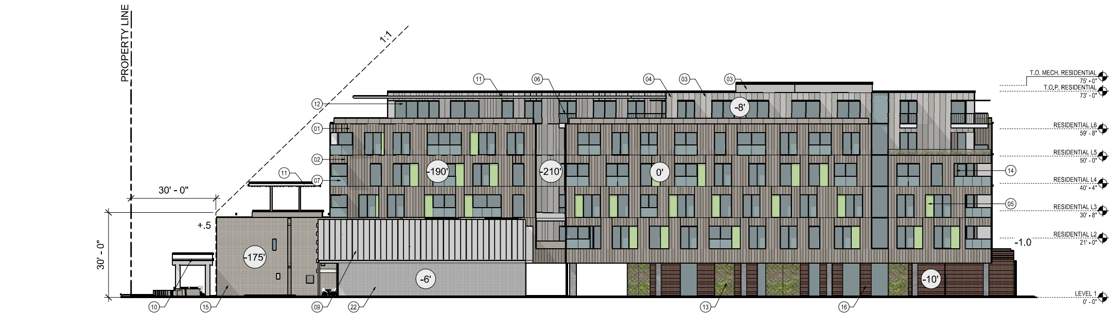
01 ELEVATION - RESIDENTIAL EAST SCALE: 1/16" = 1'-0"
