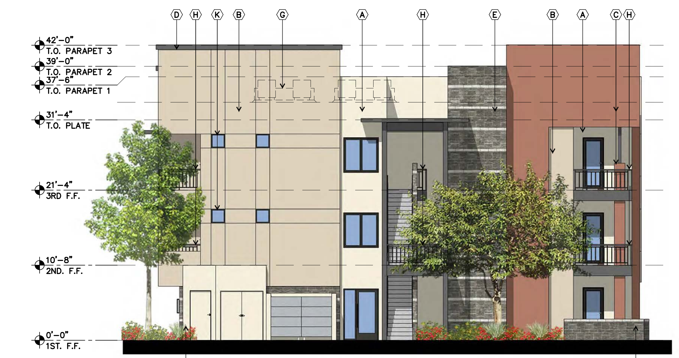
3 BUILDING 3 - RIGHT SIDE ELEVATION SCALE: 1/8" = 1'-0"
