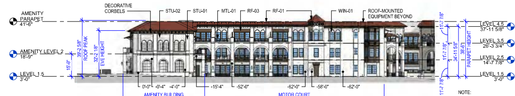
3 NORTH ELEVATION - AMENITY BUILDING - DRB 1" = 20'-0"
