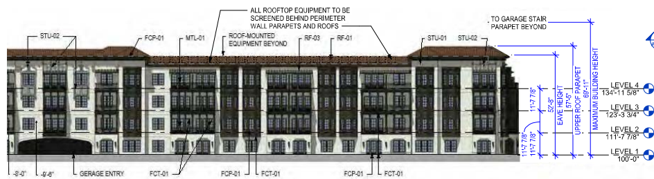
4 PARTIAL WEST ELEVATION 3/64" = 1'-0"
