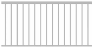
RLG.1 METAL RAILING, PAINTED LOCATION: RESIDENTIAL UNIT BALCONIES PRODUCT EXAMPLE: PICKET RAILING, FLOOR MOUNTED FINISH: PEARL LIGHT GREY POWDER-COATED, RAL 9022 MANUFACTURER: ENDURABLE BUILDING PRODUCTS
