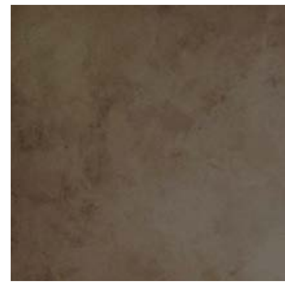
10 STC-2 - STUCCO MFG: DRYVIT OR SIMILAR, TBD BY GC TYPE: SANTA BARBARA FINISH FINISH: SEMI-SMOOTH PORTLAND CE- MENT FOR EXTERIOR SURFACES TO BE PAINTED SHERWIN WILLIAMS VAN DYKE BROWN
