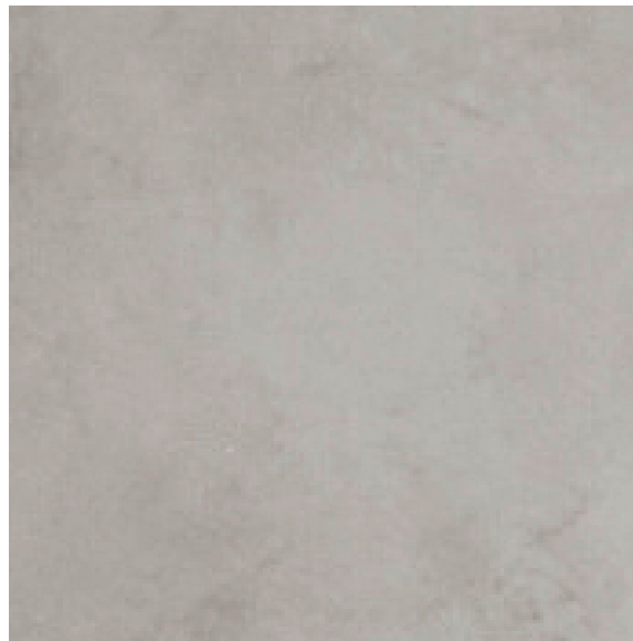
② STC-1 - STUCCO MFG: DRYVIT OR SIMILAR, TBD BY GC TYPE: SANTA BARBARA FINISH FINISH: SEMI-SMOOTH PORTLAND CEMENT FOR EXTERIOR SURFACES TO BE PAINTED SHERWIN WILLIAMS SHIITAKE
