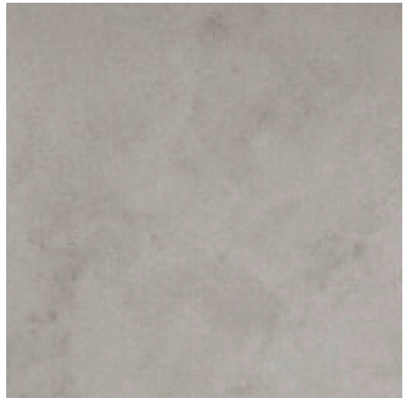
2 STC-1 - STUCCO MFG: DRYVIT OR SIMILAR, TBD BY GC TYPE: SANTA BARBARA FINISH FINISH: SEMI-SMOOTH PORTLAND CEMENT FOR EXTERIOR SURFACES TO BE PAINTED SHERWIN WILLIAMS VIRTUAL TAUPE
