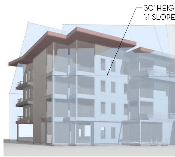
ENCROACHMENT TO SOUTH BLDG. ALONG MARSHALL WAY
