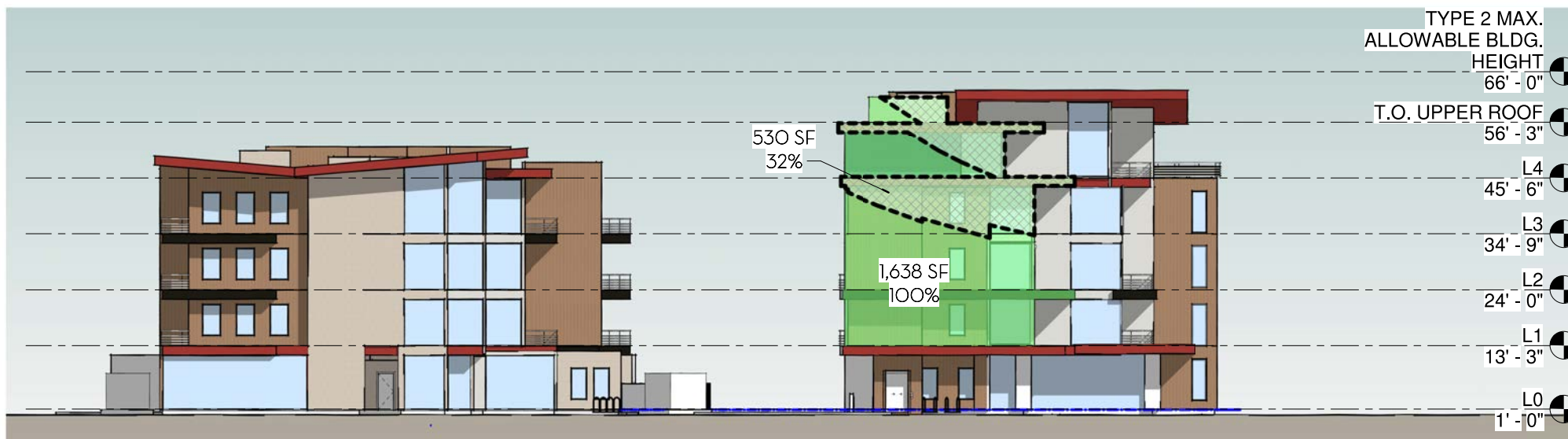
EAST ELEVATION STEPBACK ENCROACHMENT
