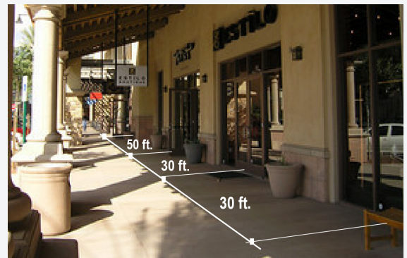
Frequent building entrances every 30-50 feet help to minimize blank walls and other dead spaces. Type 2 Development depicted.
