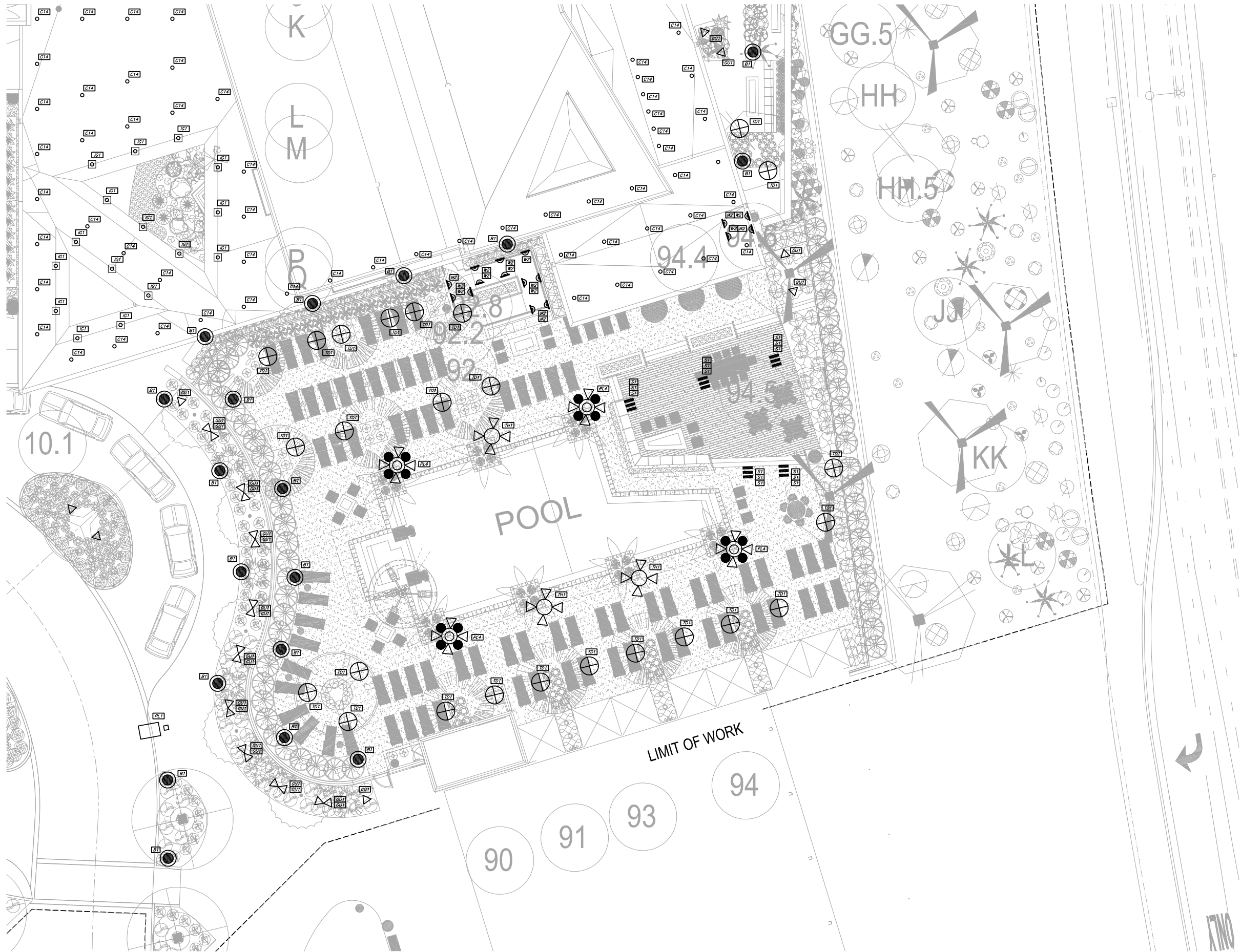
1 EXTERIOR LIGHTING PLAN - SE QUADRANT 1" = 10'-0"
