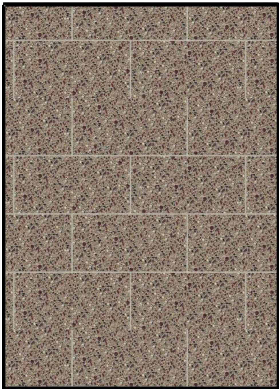
A 8"X 8"X 16" CMU BLOCK MFG: SUPERLITE BLOCK FINISH: SMOOTH FACE COLOR: MW BONE
