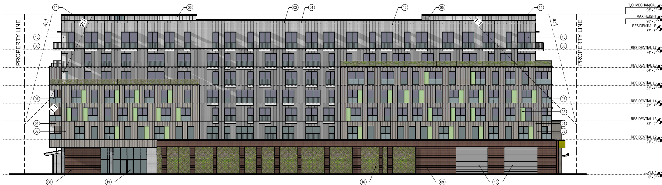
04 ELEVATION - RESIDENTIAL NORTH SCALE: 1/16" = 1'-0"
