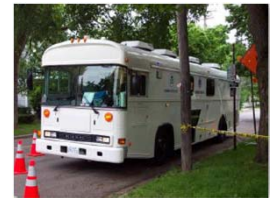
Figure 3: EPA's Trace Atmospheric Gas Analyzer Bus
