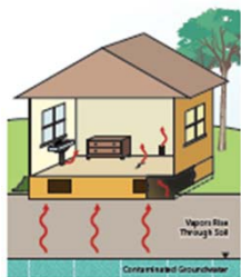
Figure 1: Vapor intrusion into a residence.
