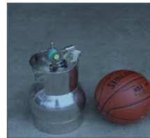
Figure 2: SUMMA Canister used for sampling indoor air
