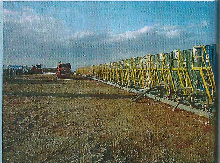
Water tanks are set up for a hydraulic fracturing job. Although this natural gas extraction technique uses relatively modest quantities of water, in some locations there already is not enough to go around.
